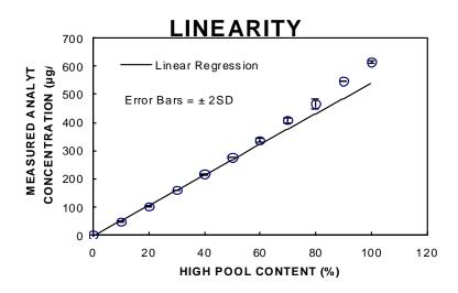
Conclusion: IRON liquicolor showed a good linearity  $>500 \,\mu\text{g/dl}$  iron measured with Hitachi 717.
