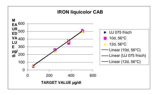
Conclusion: All results support the claimed stability of 24 months from production for the test kit.
